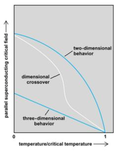
**Fig. 3** Parallel superconducting critical field versus temperature at various layer thicknesses. (*After S. T. Ruggiero, T. W. Barbee, and M. R. Beasley, Superconductivity in quasi-two-dimensional layered deposits, Phys. Rev.Lett.,* 45:1299–1302, 1980)
