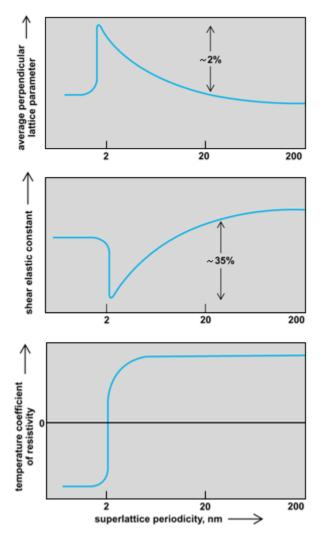
**Fig. 2** Average perpendicular lattice parameter, shear elastic constant, and temperature coefficient of resistivity versus superlattice periodicity. (*After M. R. Khan et al., Structural, elastic and transport anomalies in molybdenum-nickel superlattices, Phys. Rev., B27:7186–7193, 1983)*
